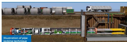
Illustration of pipe jacking technique
